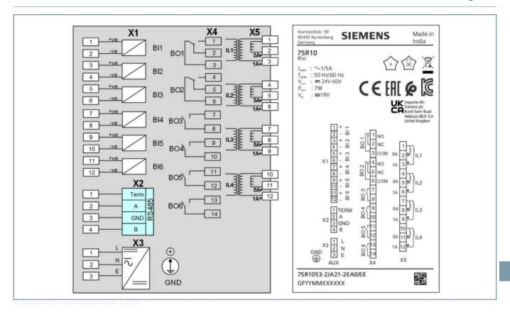
Figure 4.1/5 Terminal/Wiring Diagram of 7SR105 Non-RTD
