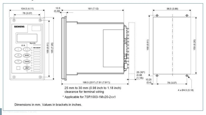
Figure 4.2/1 Front View, Side View and Panel Cut-out View
