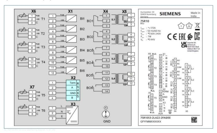
Figure 4.1/6 Terminal/Wiring Diagram of 7SR105 RTD
