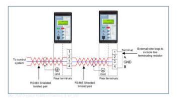
Figure 3.3/1 Typical RS485 Connection
