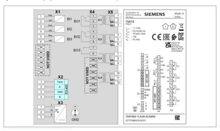
Figure 4.1/2 Terminal/Wiring Diagram of 7SR10 Non-Directional Overcurrent Relay (3 BI, 3 BO)
