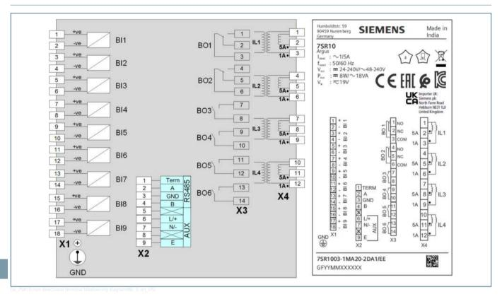
Figure 4.1/3 Terminal/Wiring Diagram of 7SR10 Non-Directional Overcurrent Relay, Universal Power Supply
