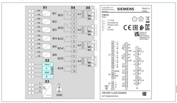
Figure 4.1/1 Terminal/Wiring Diagram of 7SR10 Non-Directional Overcurrent Relay
