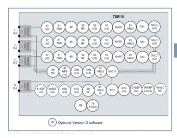
Figure 2.2/2 7SR10 Non-Directional Overcurrent Relay
