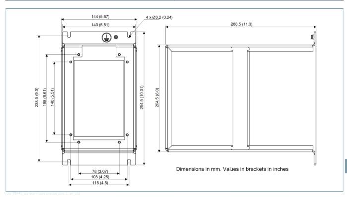
Figure 4.2/4 Front and Side Views Surface Mounting Bracket Dimensions and Panel Cut-out
