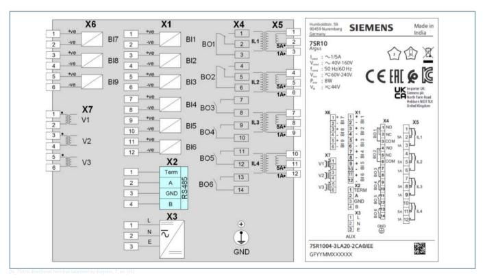
Figure 4.1/4 Terminal/Wiring Diagram of 7SR10 Directional Overcurrent Relay
