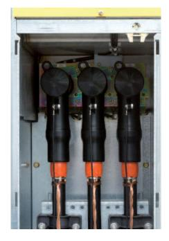
Raychem screened separable connectors RSTI-58 are designed to connect single- and three-core polymeric cables to medium-voltage gasinsulated switchgear and other equipment using CENELEC bushings type "C" specified for 630/1250 A up to 24 kV. Made of
