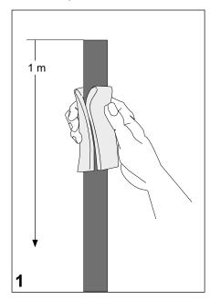
Clean and degrease the end of the oversheath for a length of 1 metre with solvent wipe.
