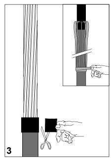
Wrap one turn of sealant tape (grey) with no overlap and slight tension around the end of the oversheath.
