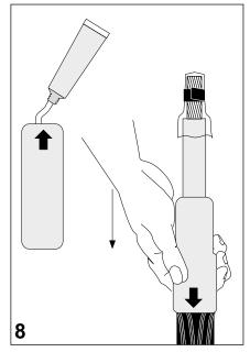
Apply onto the inner surface of the stress cone at the bottom end a 3 cm long sausage of assembly lubricant and spread it evenly over the inner surface. Use assembly lubricant without sponge top. Push the stress cone in one sequence with a twisting movement over the assembly aid completely onto the insulation until the inner collar of the stress cone stops at the oversheath cut back of the cable.
