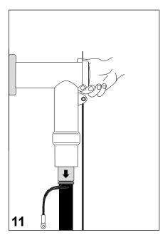
Remove from the installed connector the conductive endcap and save it in a clean container.
