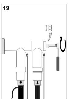
Clean the inner surface of connector back end and apply a thin layer of assembly lubricant. Do the same with the conical interface of the back plug as shown in detail.
