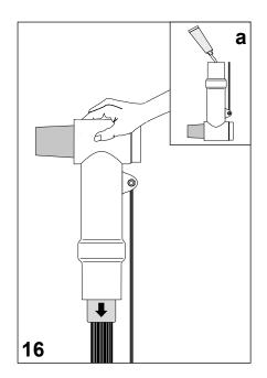
Clean the coupling connector body at the bottom end and apply a thin layer of lubricant onto the inner surface without the sponge top as shown in detail **a**.
