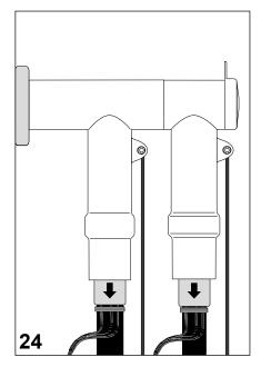
Screened separable coupling connector completed.
