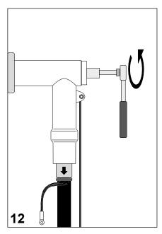
Remove from the installed connector the back plug and save it in a clean container.
