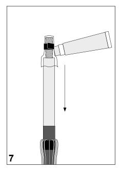
Slide the small protective bag (assembly aid) over the exposed conductor and tie it down with a PVC tape as shown in the drawing.
