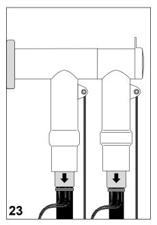
Ensure that the grounding lead is fastened tightly.
