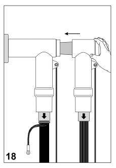
Align the conical front end of the coupling connector with the rear end of the already installed connector and push the coupling connector in position.
