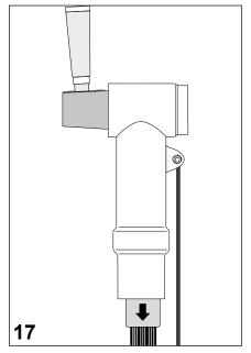
Clean the conical front end of the coupling connector and apply a thin layer of lubricant onto the outer surface of the cone with the sponge top.
